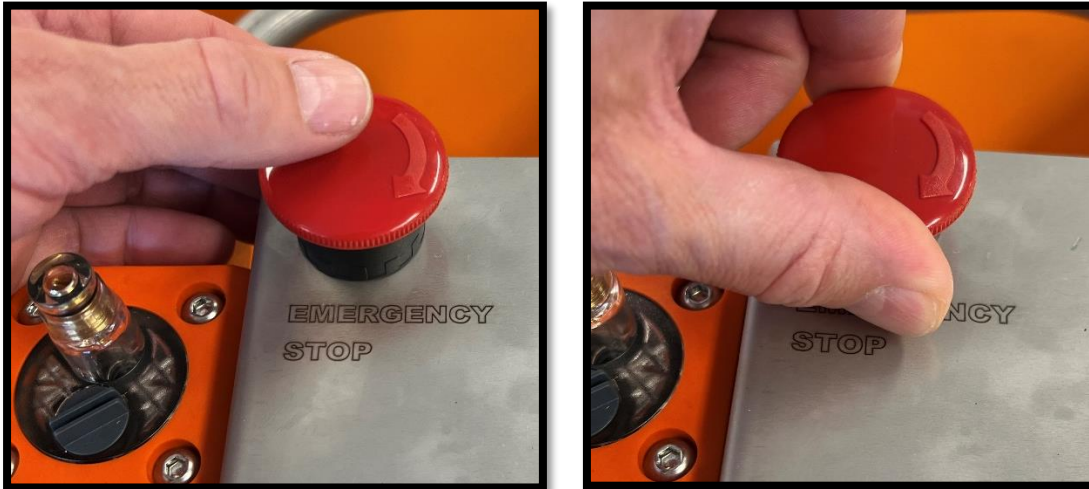
Fig.5: Images showing releasing of emergency stop switch.
