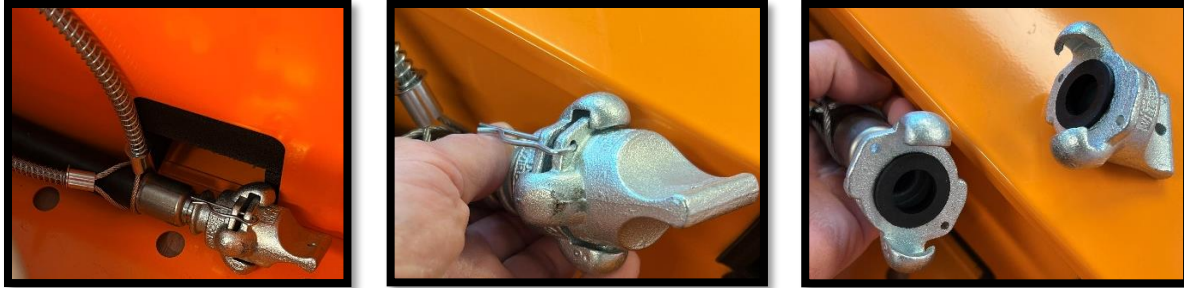
Fig.3: Images showing the Chicago claw end on the inlet pipe.
