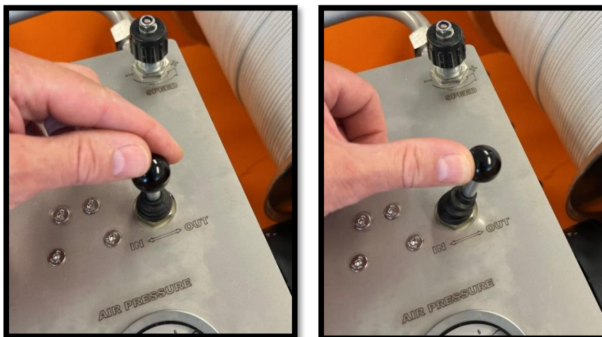
Fig.6: Control lever on the winch for spool in and out.
