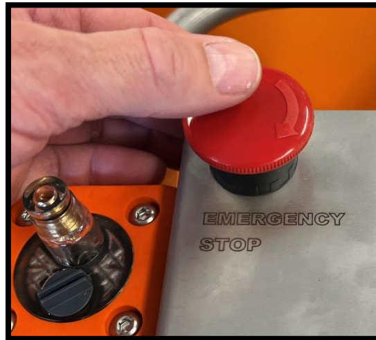
Fig.9: Image showing emergency stop switch.
