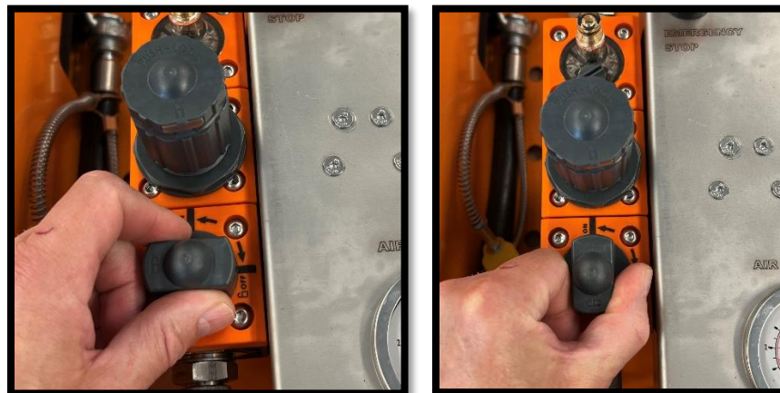
Fig.4: Images showing turning ON the main air inlet valve.
